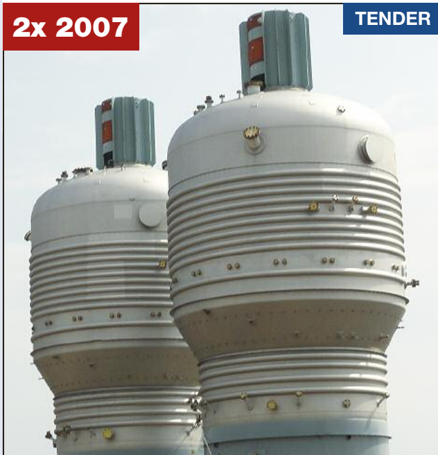
oxidative esterification reactors Kobelco JCWSA-100163 - cap. 218.460 l
